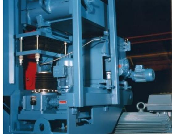
Patented band strain system. Automatic strain control and adjustment system.
